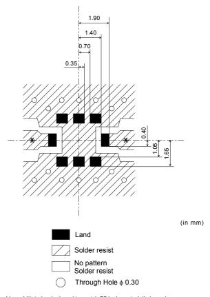
\*Line width to be designed to match  $75\Omega$  characteristic impedance, depending on PCB material and thickness.
