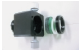
2. Insert, in order, the optical filter, spacer ring and retaining ring.
