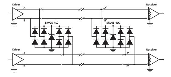
When operated in a differential mode (I/O to I/O) configuration, the SRV05-4LC has a typical device capacitance of 0.7pF. In a common mode configuration (I/O to ground), the capacitance rises to 1.4pF. In either case, the SRV05-4LC can handle up to 1Gbps data rate without any observable depreciation in signal integrity.
